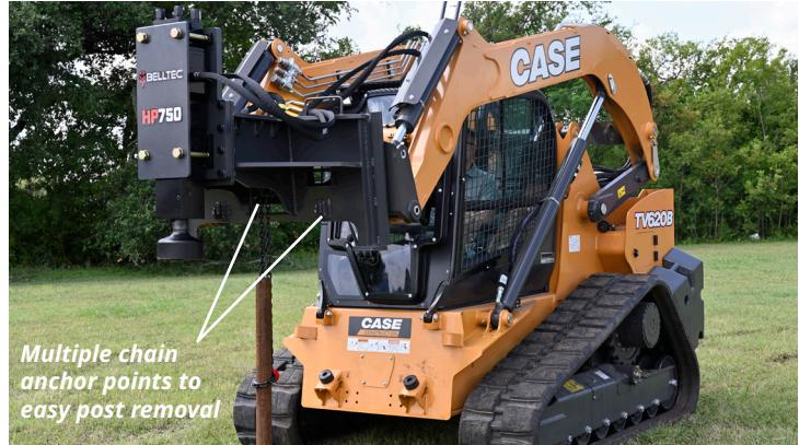
The operator is in full control of the post during the installation. Vertical accuracy can be adjusted on the fly using the domed cup drive tool to ensure the post is straight, and the pulling chain serves as a depth gauge and plumb bob.
