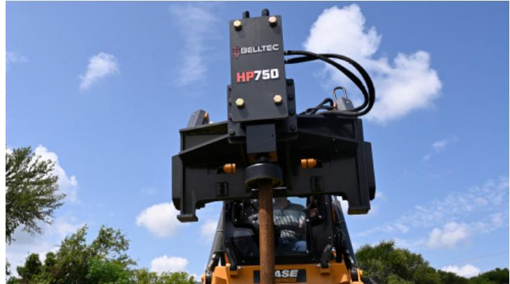
The HP750 accommodates several styles of posts, including wood, and steel pipe. The robust frame is designed for the toughest ground conditions and the power cell can be mounted on a skid loader or excavator.
